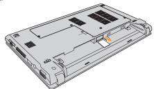
**6** Put the battery back in place. Turn the computer over and reconnect the cables.
